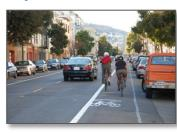
A bike lane is a portion of the roadway that has been designated specifically for bicycles by striping, signage, and pavement markings. Bike lanes enable bicyclists to ride at their preferred speed without interference from prevailing traffic conditions and facilitate predictable behavior and movements between bicyclists and motorists (NACTO). Bicycle lanes are typically best used on major roads, provide direct access to key areas, and include one-way travel.
