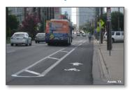
Buffered bike lanes are conventional bicycle lanes paired with a designated buffer space separating the bicycle lane from the adjacent motor vehicle travel lane and/or parking lane (NACTO).
