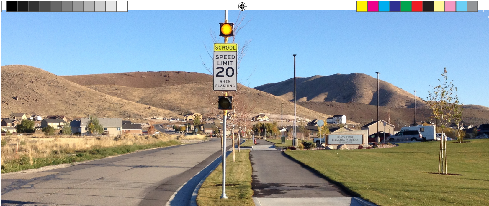
School zone speed limit sign and yellow flashing beacons in front of Black Ridge Elementary School
