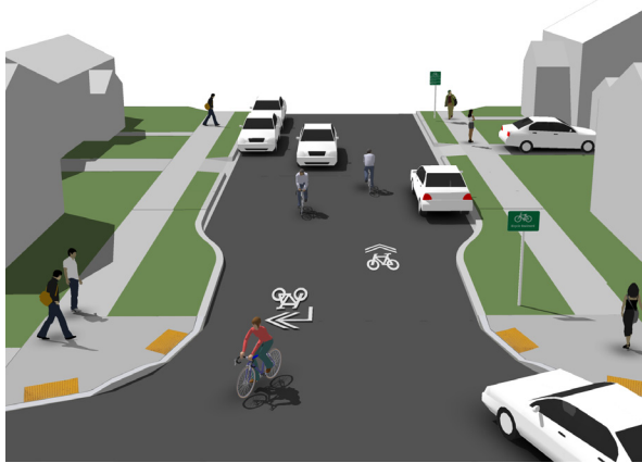
Bicycle boulevard treatments shown include wayfinding signage, directional wayfinding pavement markings, and curb extensions
