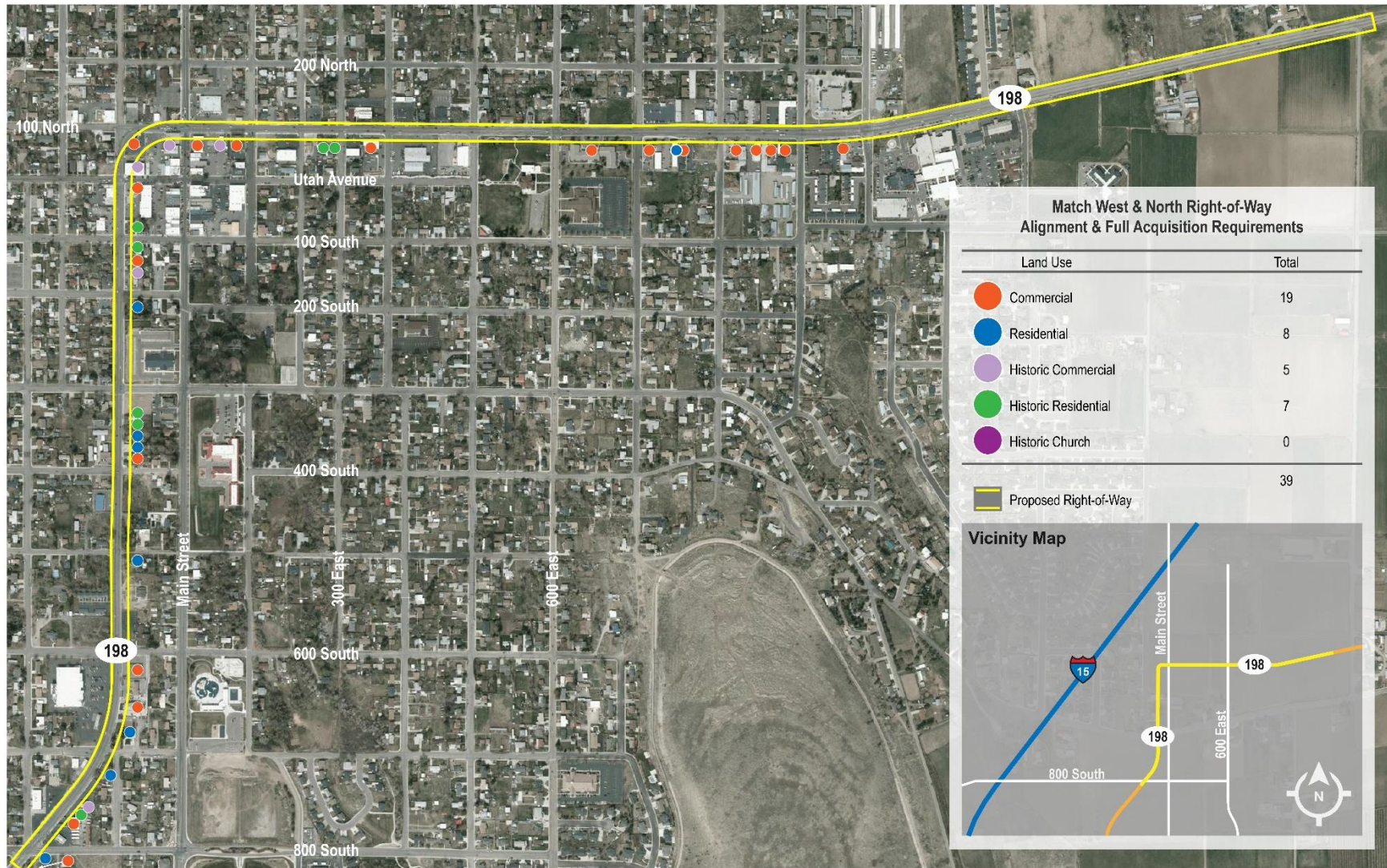
Figure 3-12: Match West and North Right-of-way
