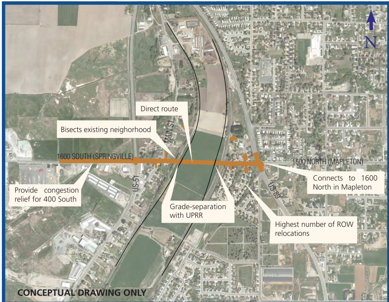
Figure 3.4-5, Alternative B1: Current Master Plan Alternative, straight connection from Springville 1600 South to Mapleton 1600 North
