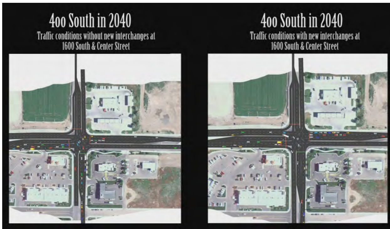
Figure 2-2, This side-by-side microsimulation of 400 South was shown to the public to demonstrate traffic conditions on 400 South with and without the interchanges evaluated in this study
