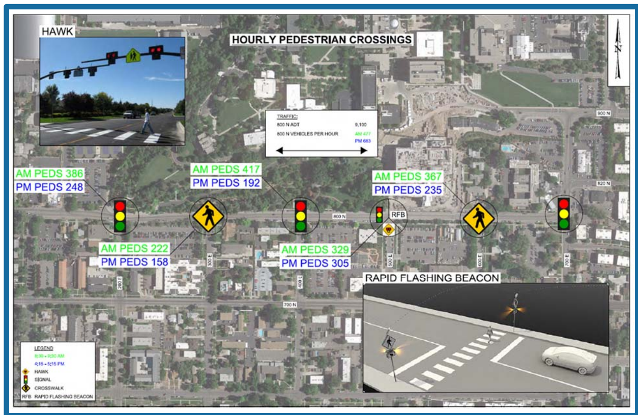
Figure 46. Recommended pedestrian crossings on 800 North.
