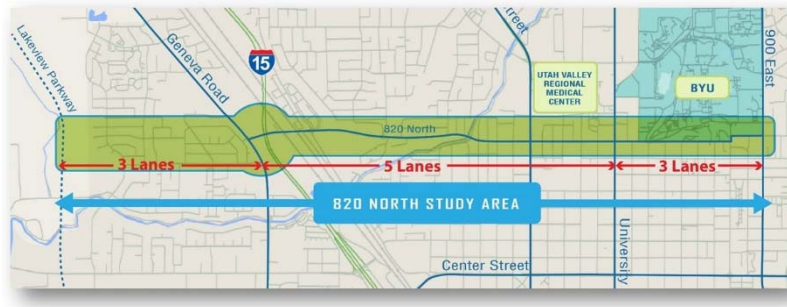
Figure 17. Travel Lane Requirements
